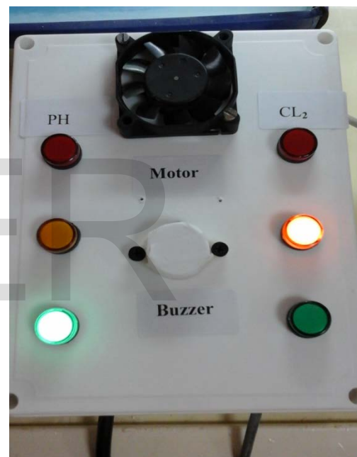
Fig.4 The output control signals
